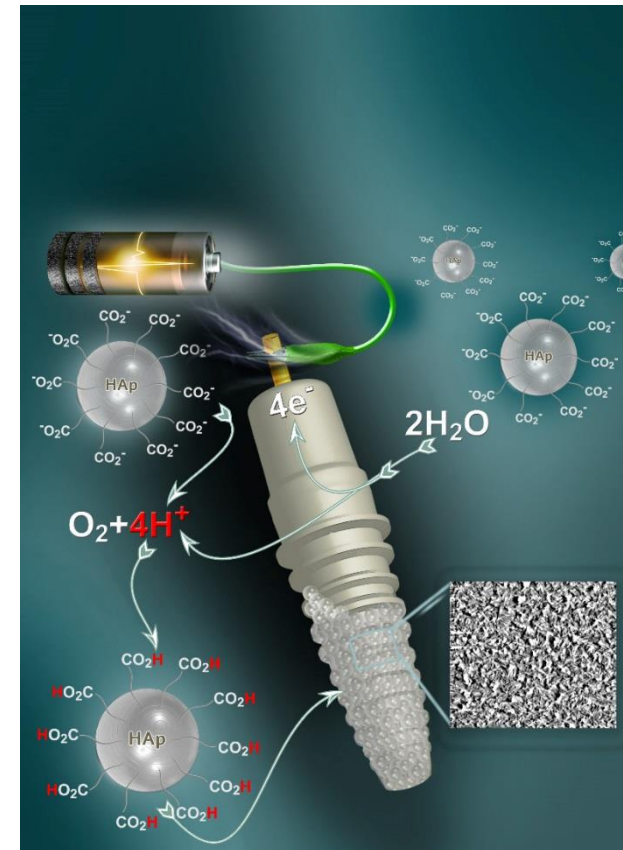
dental implant electrodeposited with HAp NPs stabilized by Cit at 2 V for 25 min
