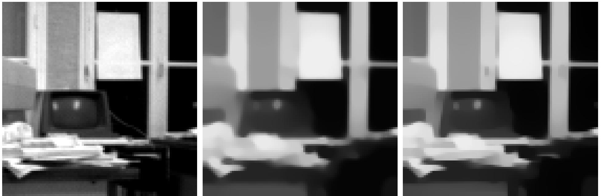
Comparison of schemes for TV diffusion. **Left:** Original image,  $93 \times 93$  pixels. **Middle:** Standard explicit scheme for regularised TV diffusion ( $\varepsilon = 0.01$ ,  $\tau = 0.0025$ , 40000 iterations). **Right:** Same with LAS scheme without regularisation ( $\tau = 0.1$ , 1000 iterations). Note that 40 times larger time steps are used.
