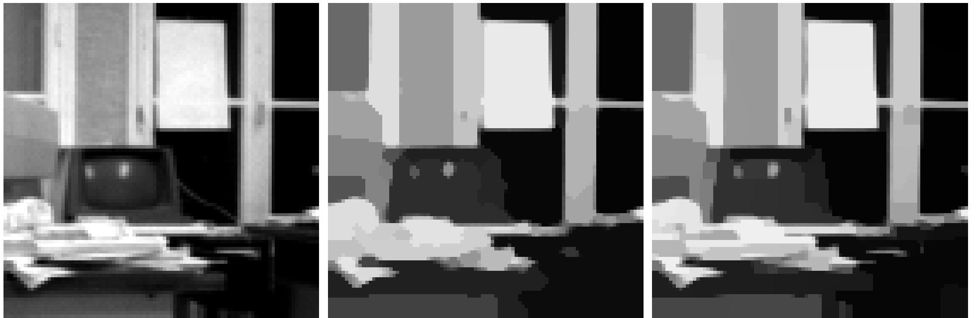
Comparison of schemes for BFB diffusion. **Left:** Original image,  $93 \times 93$  pixels. **Middle:** Standard explicit scheme for regularised BFB diffusion ( $\varepsilon = 0.1$ ,  $\tau = 0.0025$ , 160000 iterations). **Right:** Same with LAS scheme without regularisation ( $\tau = 0.1$ , 4000 iterations). Note that 40 times larger time steps are used.
