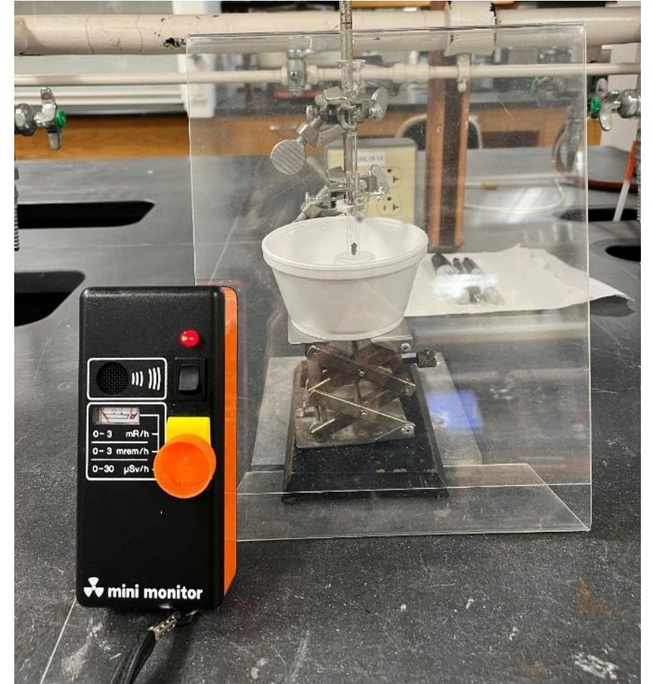
Filling apparatus behind plexiglass shield
