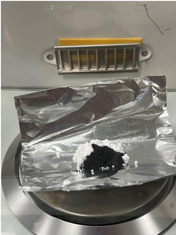
Black uranium oxide mixed with organic substrate
