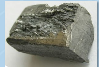
Highly pure, Ca-reduced Tb-metal. Source: Reade Advanced Materials.
