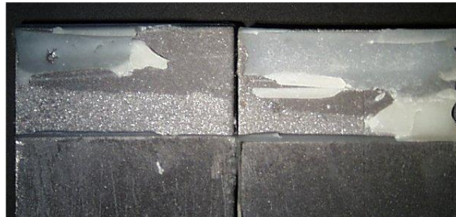
b1) -40°C-mixed mode failure
