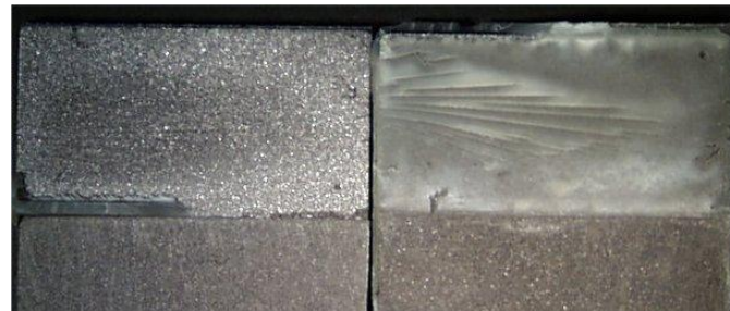
c) 80°C - adhesive failure
