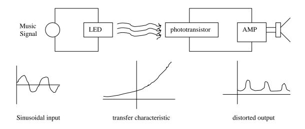
Description: Nonlinear resistors, diodes, load line analysis, small signal.
