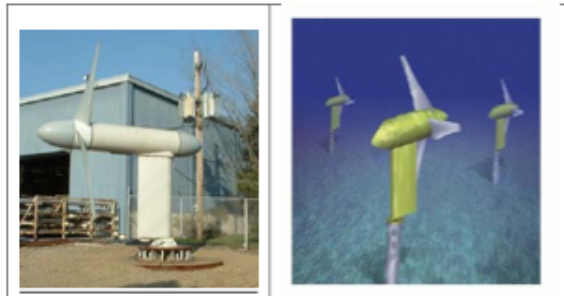
Figure 121. Verdant Power RITE Turbines
