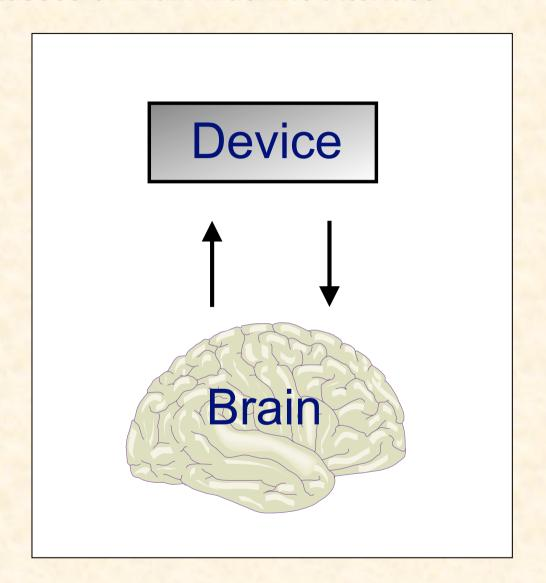
A brain-machine interface can be broadly defined as a device which interacts directly with the nervous system, bypassing the usual sensory or motor modalities.
