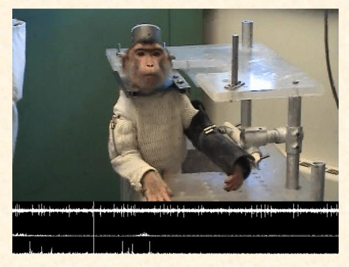
Neural signal from primary motor cortex and EMG from two wrist muscles recorded to on-board memory during reach-and-grasp movements.
