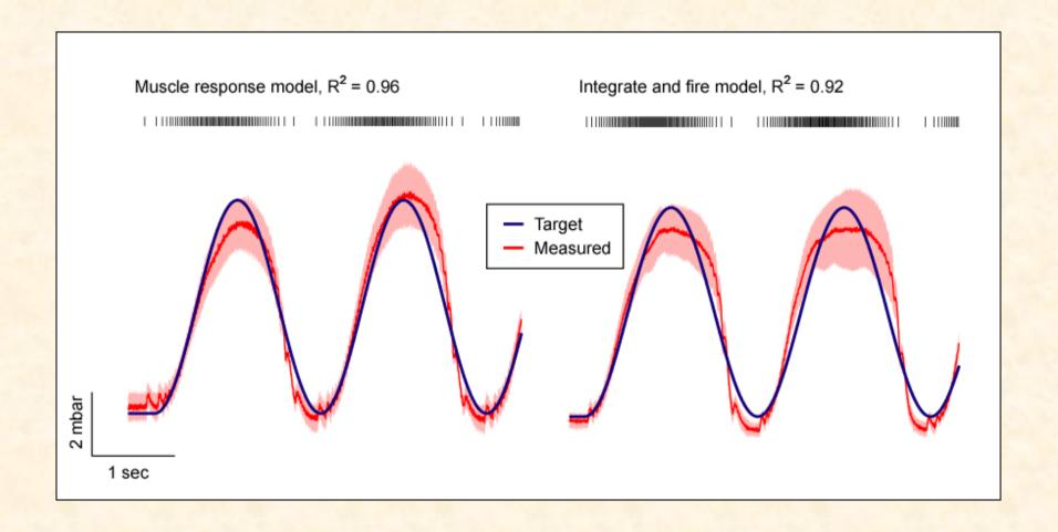
Measured grip force in response to cISMS trains closely matches a variety of target force functions.
