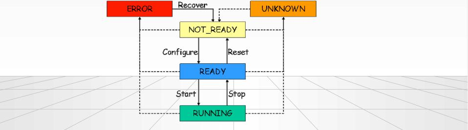
LHCb DAQ /Trigger Finite State Machine diagram (simplified)
