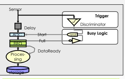
The system is busy during the ADC conversion time + processing time until the data is written to the storage
