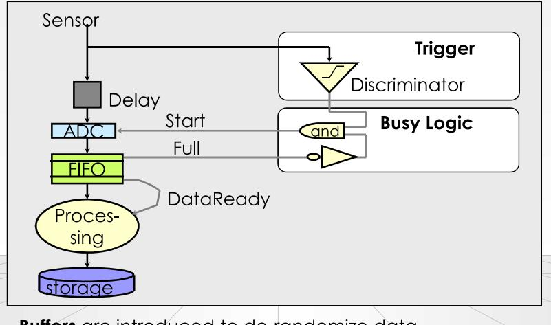
**Buffers** are introduced to de-randomize data, to decouple the data production from the data consumption. **Better performance**.
