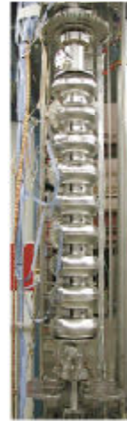
60mm-Aperture Re-Entrant Cavity, 58 MV/m! KEK/Cornell Collaboration
