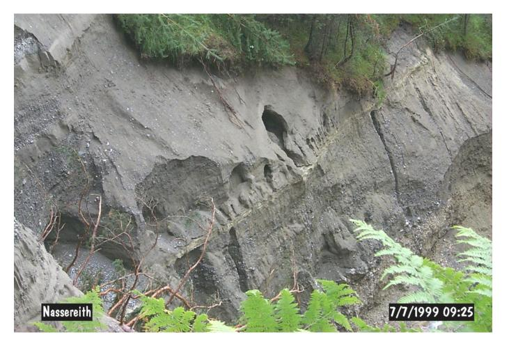
Suffosion holes in glacial sediments due to seeping water, weakening the stability of the slope
