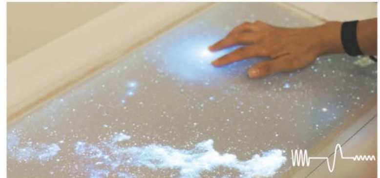
Figure 12: A visual star field in concert with a tactile layer conveying radiation intensity.
