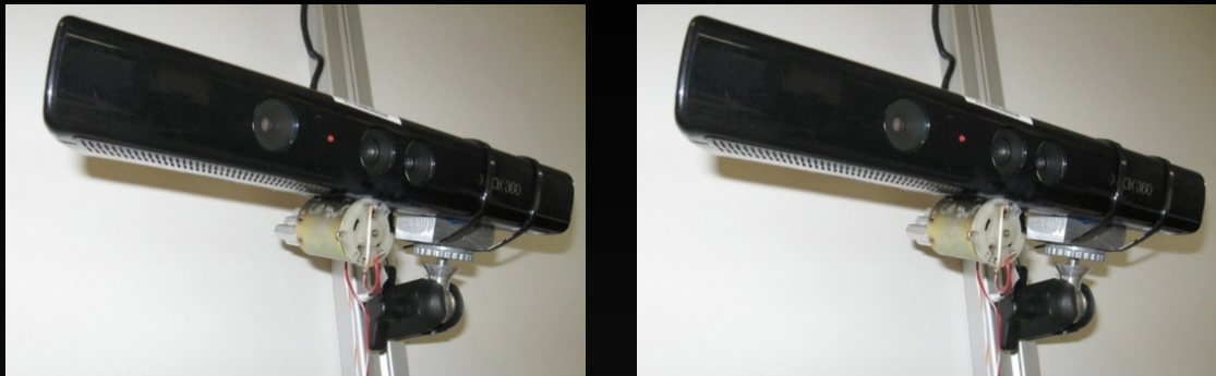
Kinects fitted with DC motors with eccentrics
