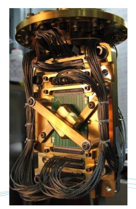
and system cooled to 20mK in a magnetically shielded environment (50000x smaller than earth's magnetic field)
