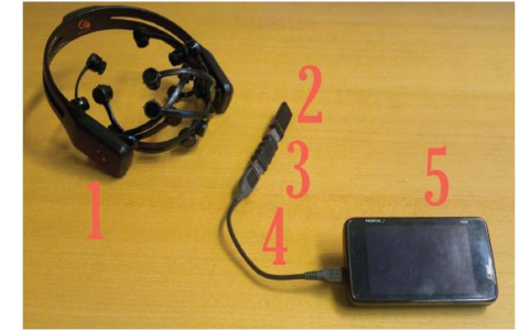
Fig. 1. Handheld brain scanner components. Emotiv EPOC wireless EEG headset (1), Emotiv Receiver module with USB connector (2), USB connector and adapter (3+4), and Nokia N900 mobile phone. The total cost of the system is less than USD1000.
