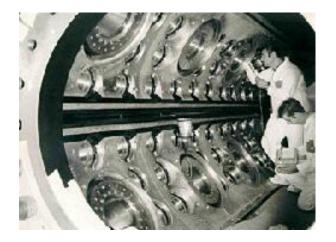
Gargamelle, a very large heavy-liquid (freon) chamber constructed at Ecole Polytechnique in Paris, came to CERN in 1970. It was 2 m in diameter, 4 m long and filled with Freon at 20 atm.
