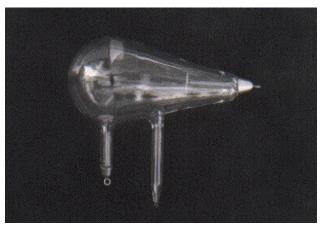
This tube is a glass bulb with positive and negative electrodes, evacuated of air, which displays a fluorescent glow when a high voltage current is passed though it. When he shielded the tube with heavy black cardboard, he found that a greenish fluorescent light could be seen from a platinobaium screen 9 feet away. Conrad Röntgen discovered X-Rays in 1895.
