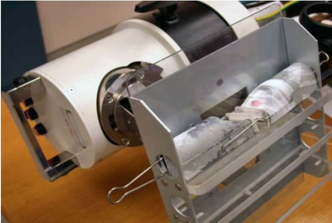
Setup of tumour irradiation – shielding of the body, while only tumour is exposed to irradiation
