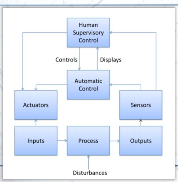
Basic control loop in the control rooms of modern process industries
